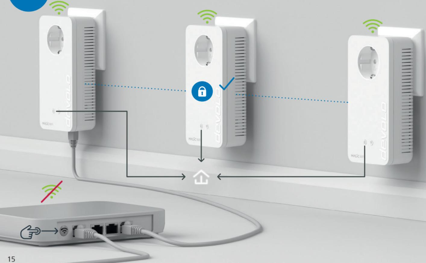
**| EN |** Once the LEDs of all devices are flashing white continuously, the process is complete (a maximum of 3 minutes). Now switch off the Wi-Fi on your router (if necessary, refer to the manual for your router).
