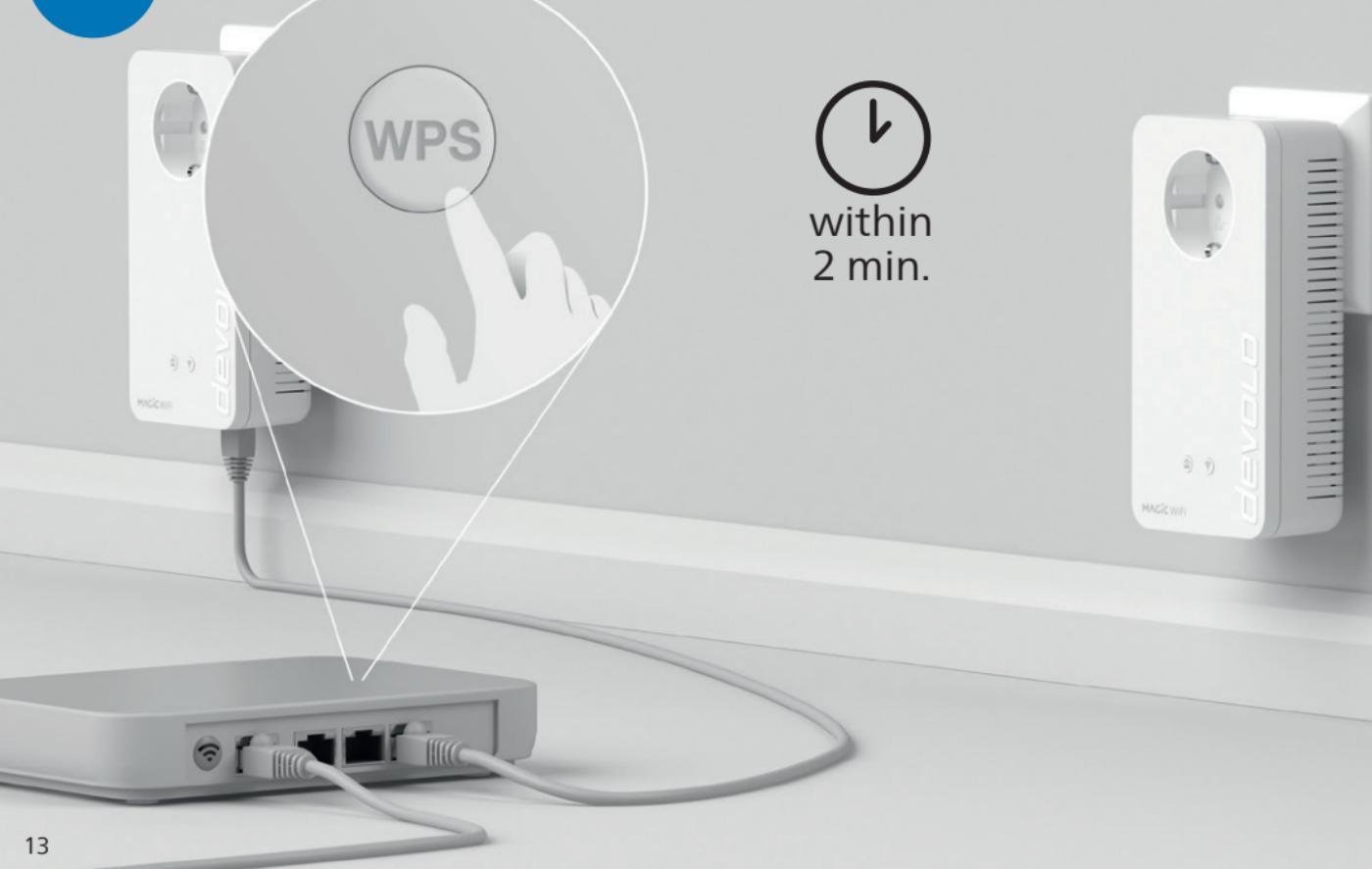
**| EN |** Within 2 minutes, press the WPS button on your Wi-Fi router. If necessary, please refer to the manual for your router to find the location of the WPS button and how long you have to press it.
